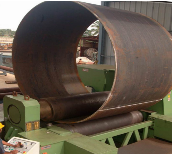
Plate Rolling Machines for cold rolling thickness up to 110mm thick x 3m width
