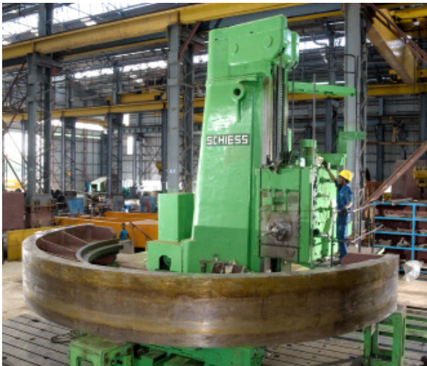
Floor Boring Machines up to 6m travel length with spindle \Phi of 130 mm
