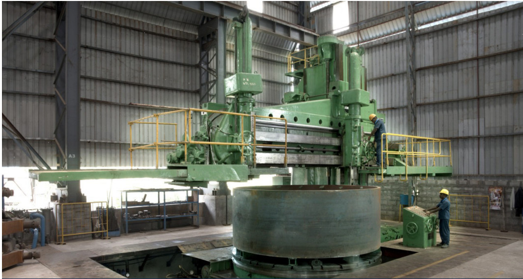
Vertical Turret Lathes with machining capacity up to 10.5m \Phi , 3m height and job weight of 100 tonnes
